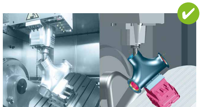
... the virtual machine enables precise simulation of the real kinematics.
